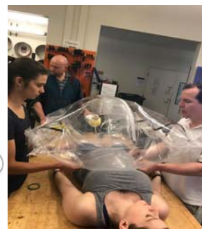
Fig. 3. Setup of ergonomic-testing rig over pregnant volunteer subject.
